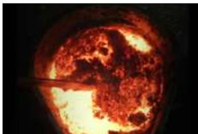
4. When melted the worthless rock becomes separated from the silver and can be scraped away
