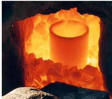
2. The rock is placed in a container called a crucible and put into the hot furnace
