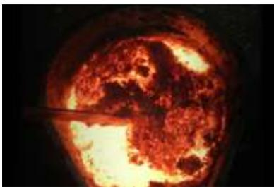
4. When melted the worthless rock becomes separated from the gold and can be scraped away
